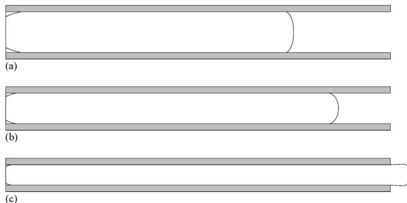
Fig. 16. Evolution of the yield surface and the material/air interface with time for Bn=10, Re=0, Ca=10^3, St=0, w=15, \epsilon=0.1, \alpha_{sl}=5, \beta_{sl}=1, N=500 at times t=0.2, t=0.4, t=0.6 .
